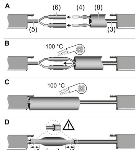
Figure 7: Linking lighting inserts
