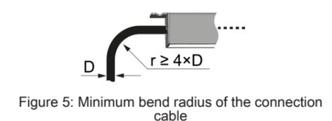
Figure 5: Minimum bend radius of the connection cable
