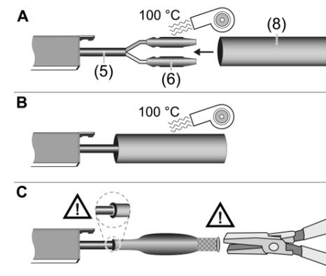
Figure 8: Sealing output cable of the last LED lighting insert
